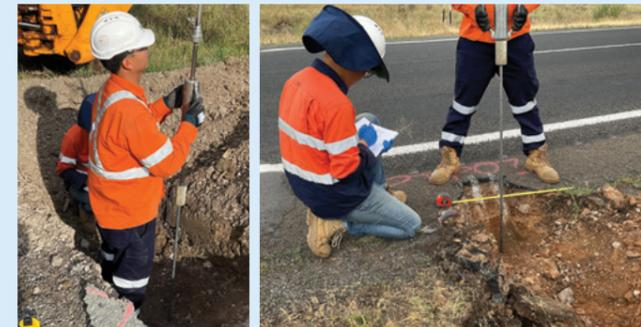
The strength of the subgrade (bottom layer of the pavement) is tested and measurements are recorded
